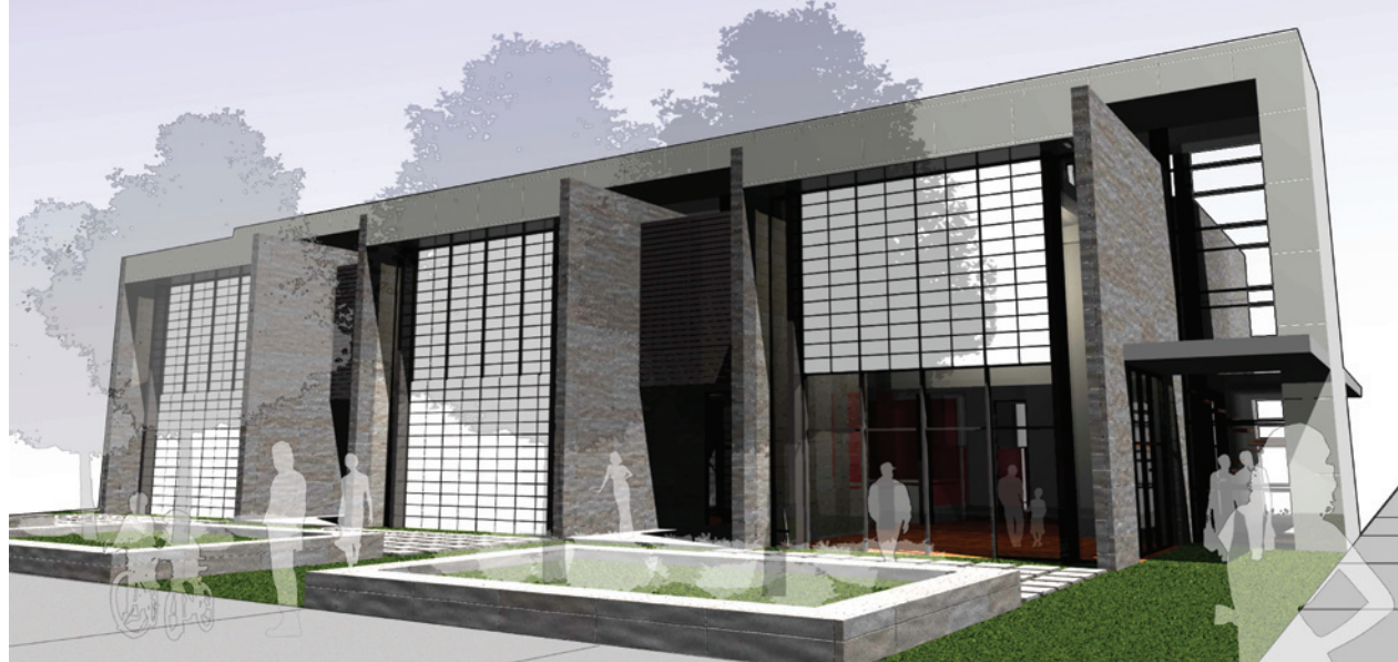
Full-height movable screen panels of reflective translucent glass over the windows bring daylight into the interior. This group's design controlled the southern sunlight and the sky-vault daylight via selective placement of glazing and the use of louver systems along with the adjustable screen panels.
