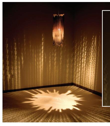
This Akari-inspired pendant, by Alexandra Ebright, measures 9" diameter x 28" high and is comprised of recycled corrugated cardboard and wire. It is lamped with a 60-watt, clear BT17 halogen.
